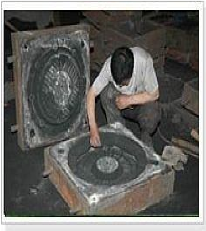
Fig. 3: A metal caster inspecting a sand mould
