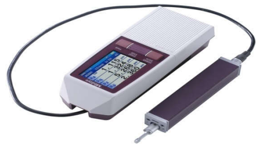
Figure 1 (a). Stylus Roughness measurement equipment
