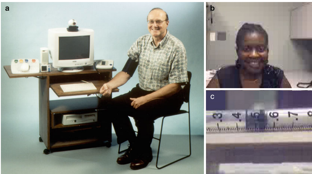
Fig. 18.3 Plain old telephone service (POTS)–based home telehealth. Panel (a) shows the IDEATel Home Telemedicine Unit. Panel (b) shows a typical full-motion video image transmitted over POTS. Because of frame-to-frame compression, images of nonmoving objects can be of even higher quality. Many home telehealth systems are
