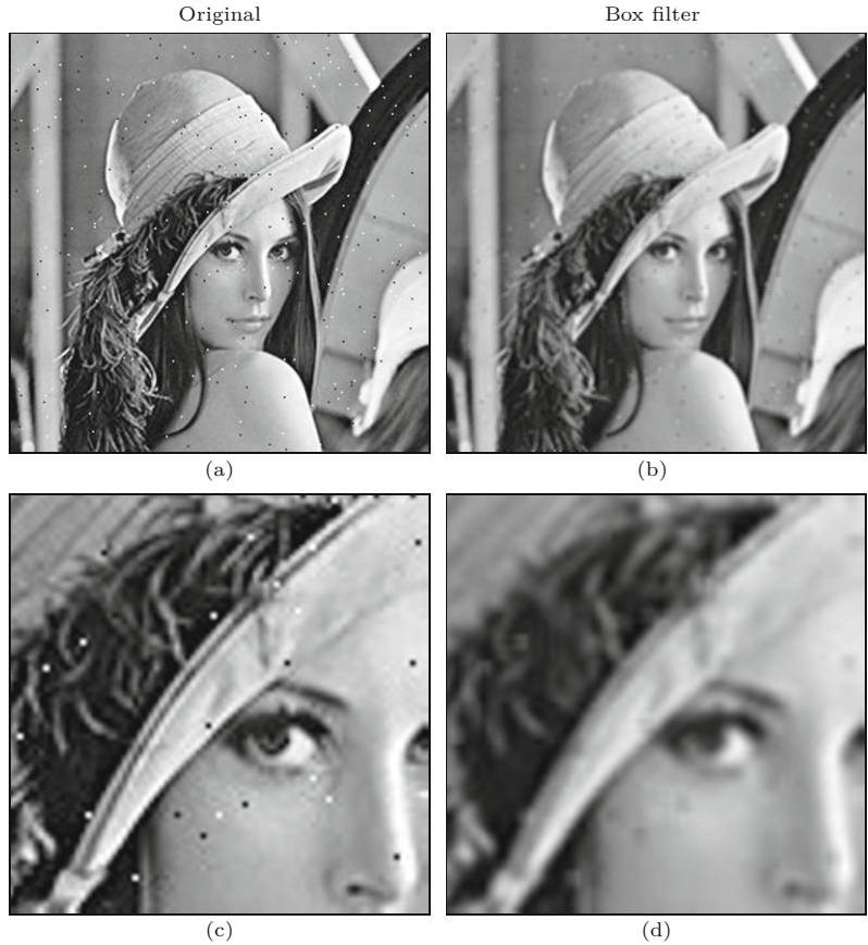
Fig. 5.14 3 \times 3 linear box filter applied to a grayscale image corrupted with salt-and-pepper noise. Original (a), filtered image (b), enlarged details (c,d). Note that the individual noise pixels are only flattened but not removed.
