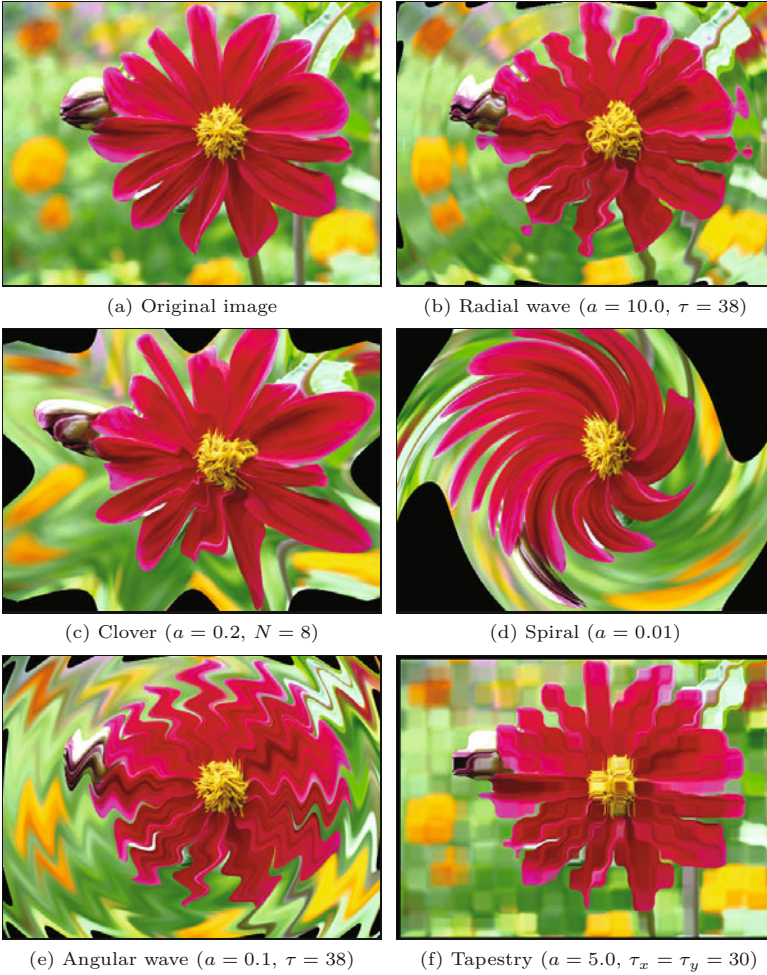
Fig. 21.11 Examples of the nonlinear geometric transformations defined in Exercise 21.4. The reference point \mathbf{x}_c is always taken at the image center.
