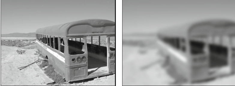
Fig. 5.1 No point operation can blur or sharpen an image. This is an example of what filters can do. Like point operations, filters do not modify the geometry of an image.
