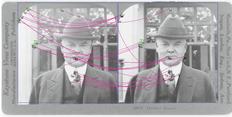
Fig. 25.31 Rejection of weak or ambiguous matches by limiting the ratio of primary and secondary match distance \rho_{\max} (see Eqs. (25.104)–(25.105)).
