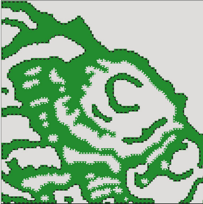
Fig. 10.11 Example of a complex contour (original image in Ch. 9, Fig. 9.12). Outer contours are marked in black and inner contours in white.
