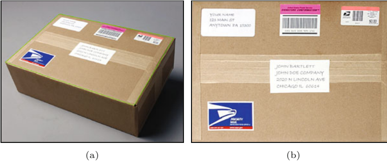
Fig. 21.12 Projective rectification example (see Exercise 21.5). Source image and user-defined selection (a); transformed output image (b).
