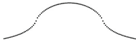
Fig. 12.23 Reconstruction by simple back projection without convolution. The object is the same as in Fig. 12.22
