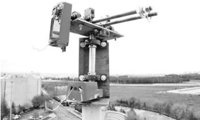
Fig. 7.14 Picture of the used two-axis dynamic system [2]
