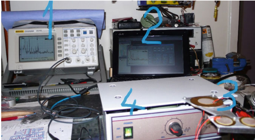
Fig. 4.3 Experiment, 1 oscilloscope, 2 data acquisition system, 3 flexible arm, 4 electronic shaker
