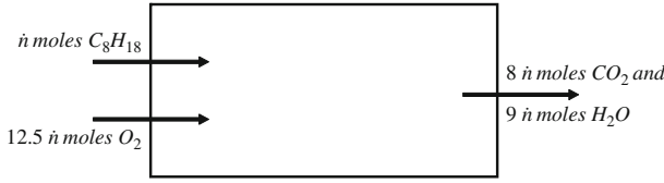
Fig. 3.13 Schematic diagram of the work production process from the chemical reaction of octane oxidation
