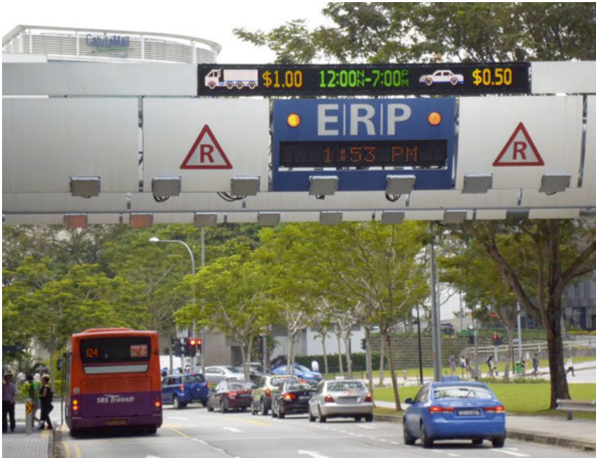
Figure 11.2 Singapore electronic road pricing system (Source: Photo taken by J. K. Lee March 2013)
