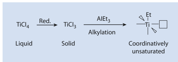
■ Fig. 11.4 Initiation process for Ziegler catalysts
