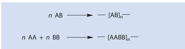
■ Fig. 8.6 A scheme of a step-growth polymerization
