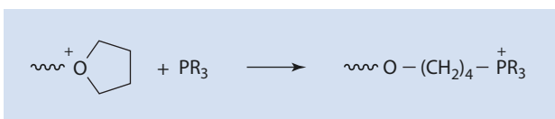
Fig. 12.26 Termination of a CROP with a phosphine to allow quantitative analysis
