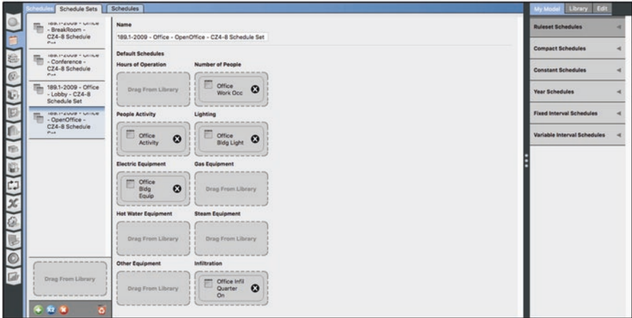
Fig. 3.2 Schedule Set for an Office Break Room
