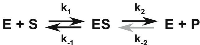
Fig. 15.1 Simplest enzyme reaction scheme for S \rightarrow P conversion invoking the formation of a single ES complex. The forward rate constants for the first and the second step are shown as k_1 and k_2 , respectively. Reverse rate constants for the corresponding steps are shown as k_{-1} and k_{-2} .
